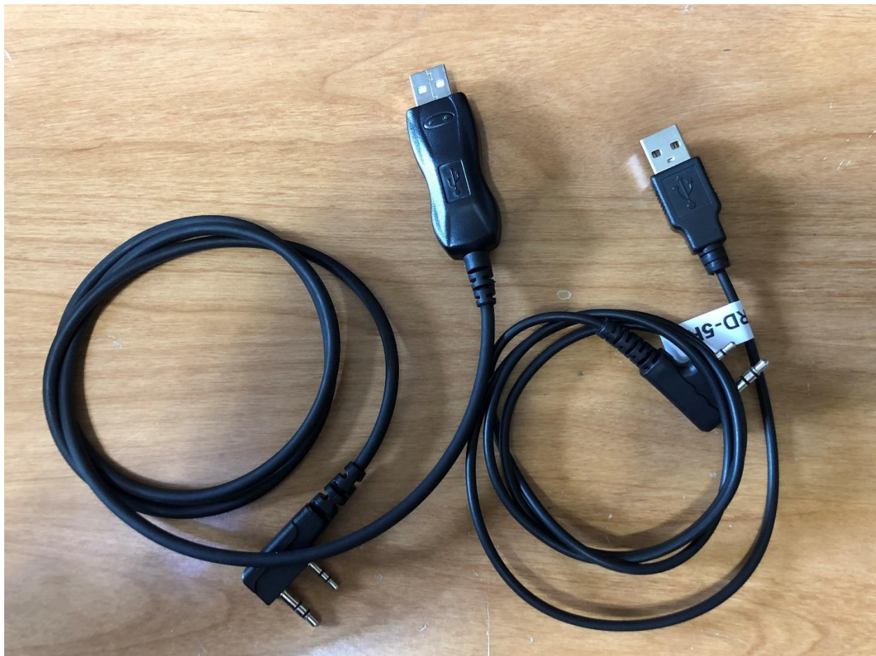
Figure 1. UV-5R programming cable (left) and RD-5R cable (right). Note how much larger is the USB connector on the UV-5R cable, because it contains a conversion chip that the RD-5R cable does not use. I labeled my RD-5R cable.
